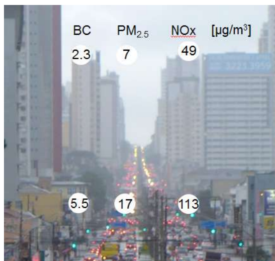
Figure 1. Mean vertical gradient of pollutants measured within a canyon street in the city center.
