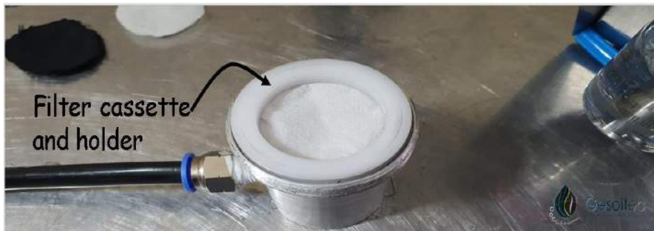
Fig 2. Filter materials were cut and placed on a filter holder for testing
